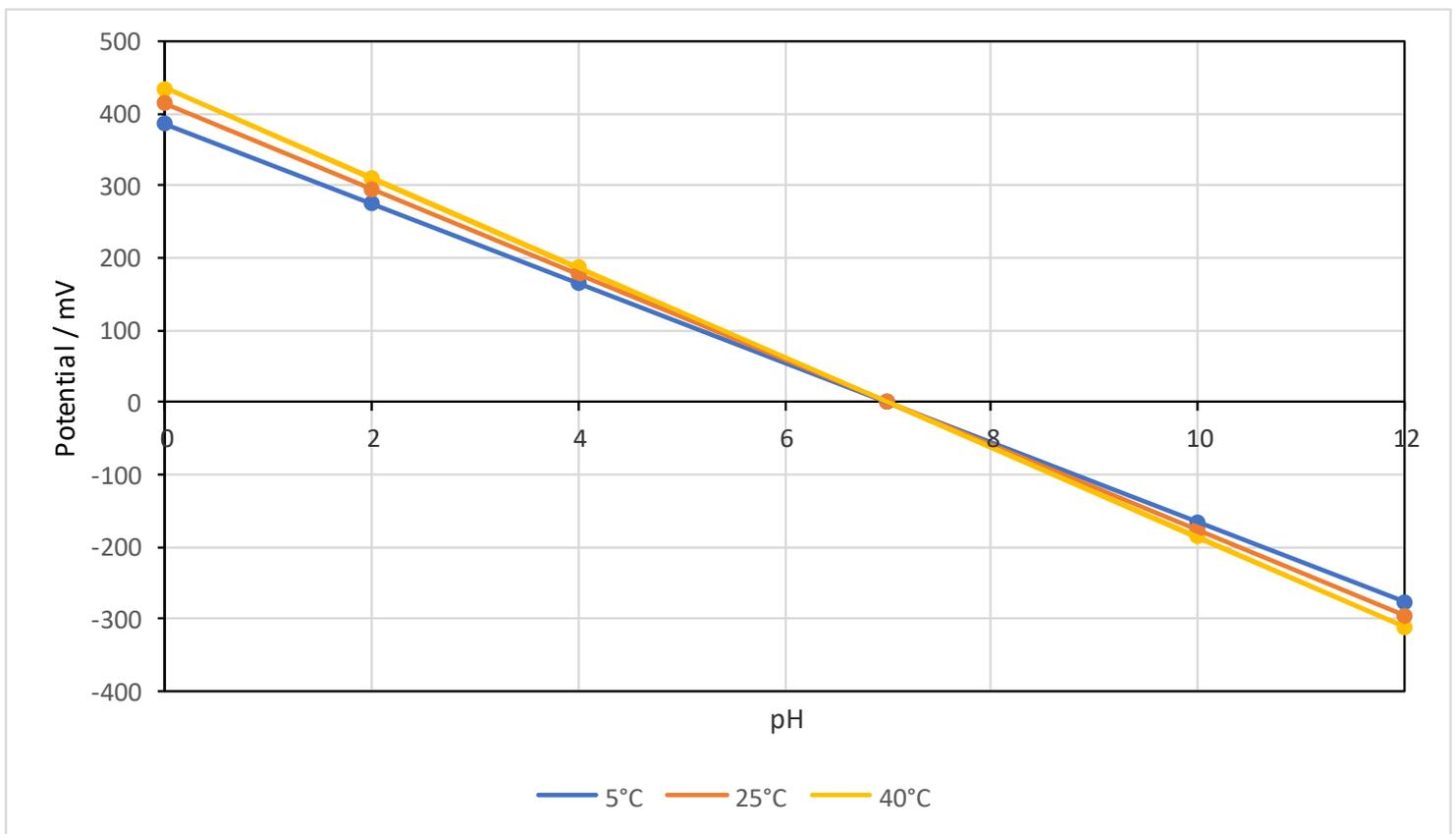
The graph above and the table below shows the pH sensor response slopes at different temperatures.
