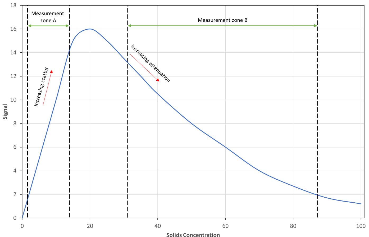
This means that a meaningful measure of TSS can be made going up the slope (measurement zone A) **and** going down the slope (measurement zone B). The problem with this is that the different samples will have a 'hump' where measurements aren't possible in different places.
